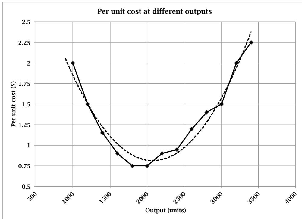
Above graph shows distribution of per unit unit cost (\$) of an automotive component at different outputs of a machine. The best estimation curve is also shown with dashed line. The following two questions are based on it.
